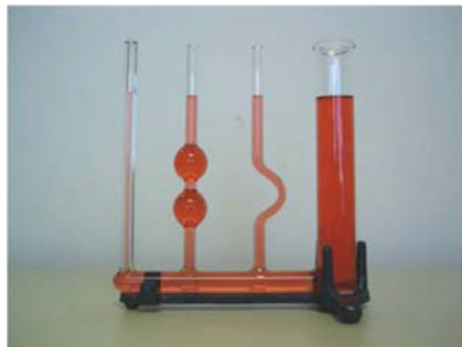
Figure 14.9 If a fluid can flow freely between parts of a container, it rises to the same height in each part. In the container pictured, the pressure at the bottom of each column is the same; if it were not the same, the fluid would flow until the pressures became equal.
